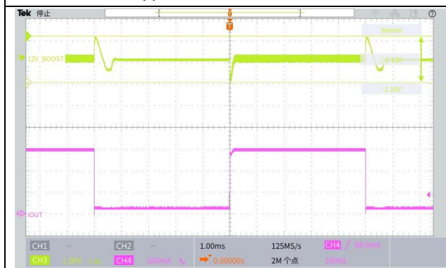
12V Load Transient, SCAP=2.5V, IOU=30mA-300mA, 0.3A/us
