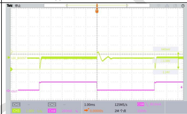
12V Load Transient, SCAP=2.5V, IOU=20mA- 200mA, 0.3A/us
