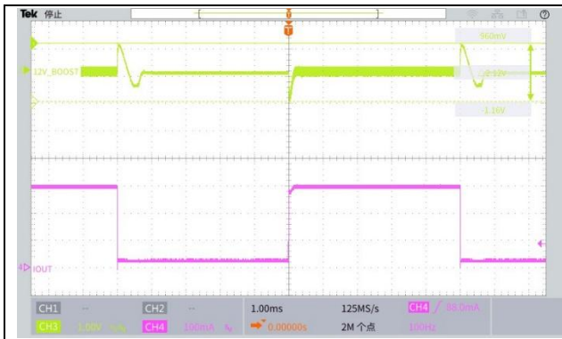
12V Load Transient, SCAP=2.5V, IOU=30mA- 300mA, 0.3A/us
